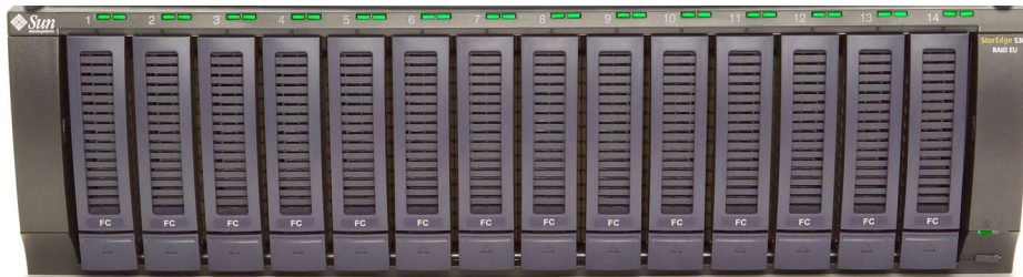
Figure 5. Front panel of StorEdge 5300 RAID Expansion Unit
