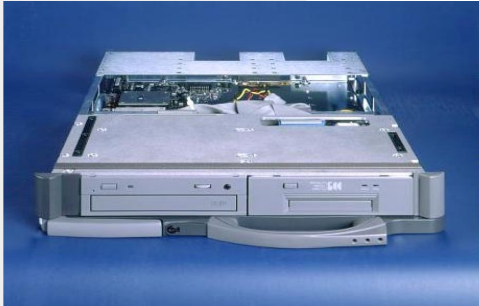
System Controller Peripheral Board
