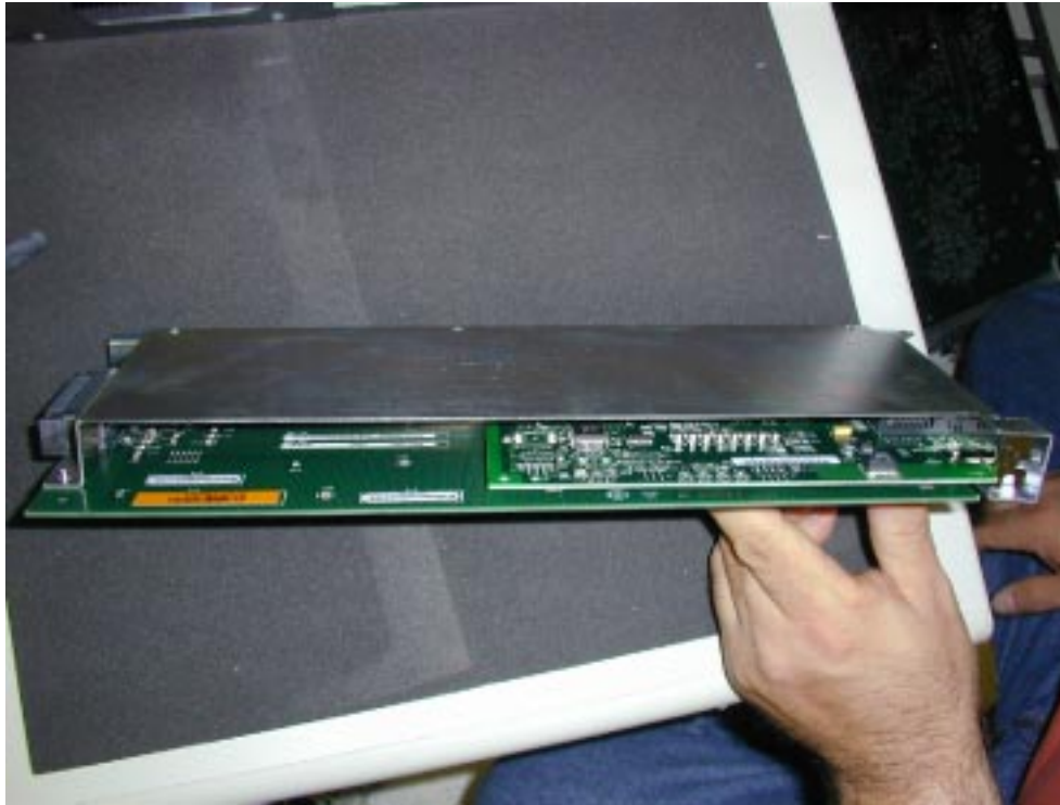
I/O Cassette with installed PCI card
