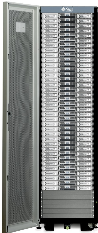
Figure 2 – Photo of Sun Fire X2250 Server installed in a rack
